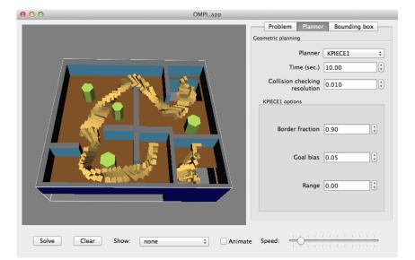
Figure 2. The OMPL.app GUI showing a path for an L-shaped robot in an office-like environment with two floors and a staircase joining them.
